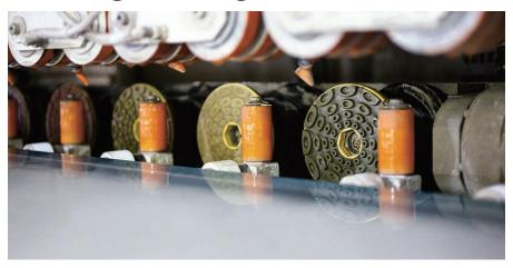
For people who has Edge Polishing Machine, we have 2 type good abrasives. One is for straight edge "TWINCUR-Resin EG2" and another is for bullnose "TWINCUR-Resin EB".
